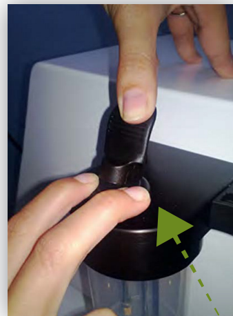
To close the bottle stopper take your index and middle finger and press down on the base of the bottle stopper. Use your thumb to press down while holding the base. Once it clicks it is secure.
